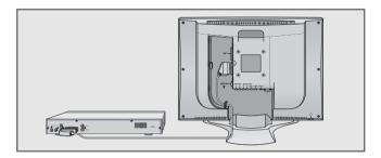
1 Connect the »AV1« or »AV2« socket (Amira 17 and 20 only) on the television and the corresponding socket on the video recorder, DVD player or the set-top box with a Euro-AV (Scart) cable.
